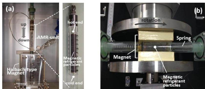
Figure 1. Pictures of (a) a primitive test apparatus of AMR-cycle and (b) a pump-less AMR-cycle system.
